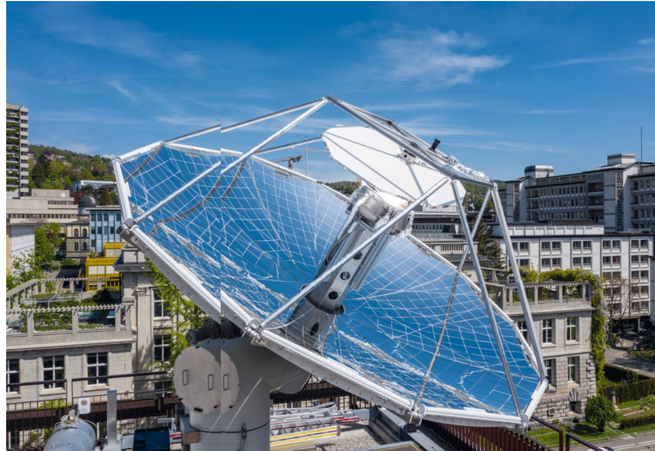
Synhelion: This mini-refinery on the roof of an ETH building produces around one decilitre of methanol a day from sunlight and air.
