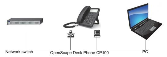
Using this connection option saves one network port for each switch used and allows shorter network cables to be used when arranged correctly.
