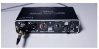
The black XLR microphone jack is inserted into  $\ll\!INPUT\,1L\!\!>$  on the front of the audio interface.
