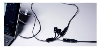
The USB splitter is connected to the Surface tablet. The grey input device and audio interface are connected to this. Following this the Surface can be started.
