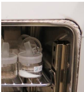
Asbestos rope seal
