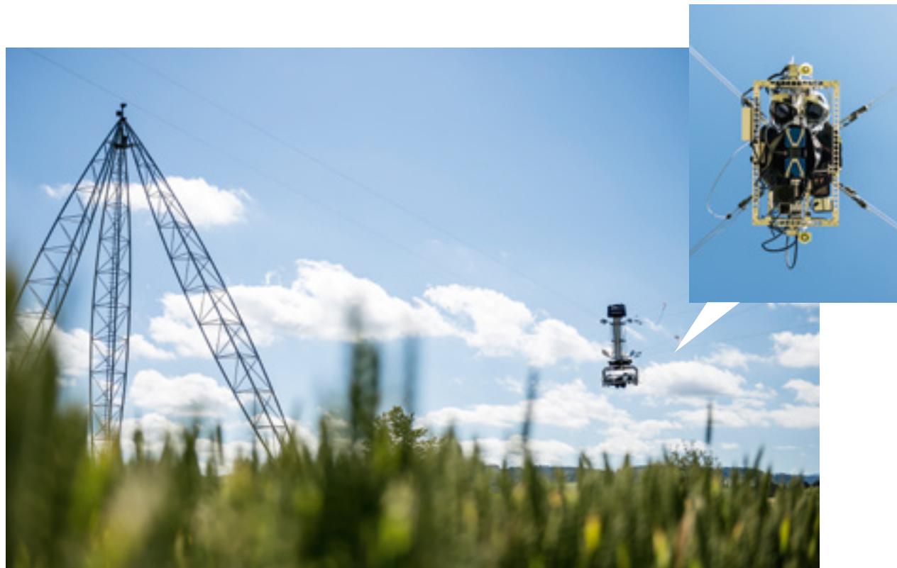
Inspired by football: The ETH researchers’ phenotyping platform is based on the principle behind the Spidercam.
