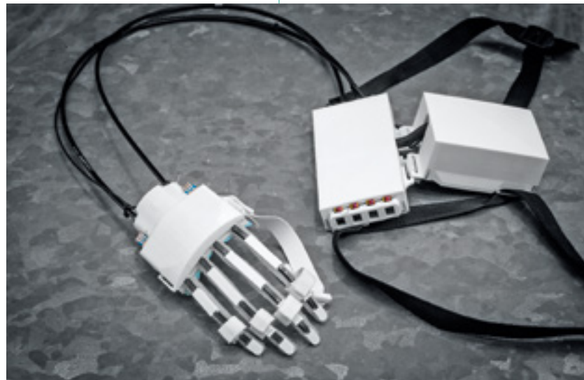
A hand exoskeleton with motors that can be fixed to the patient's back: A bicycle brake cable transmits enough force to lift a litre bottle of mineral water.
