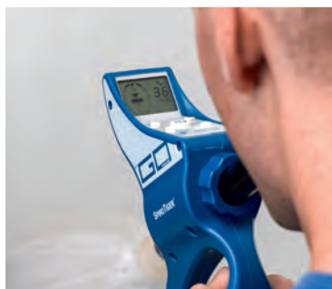
The device determines how rapidly and deeply users should breathe
