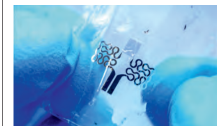
The ultra-thin temperature sensor is biodegradable
