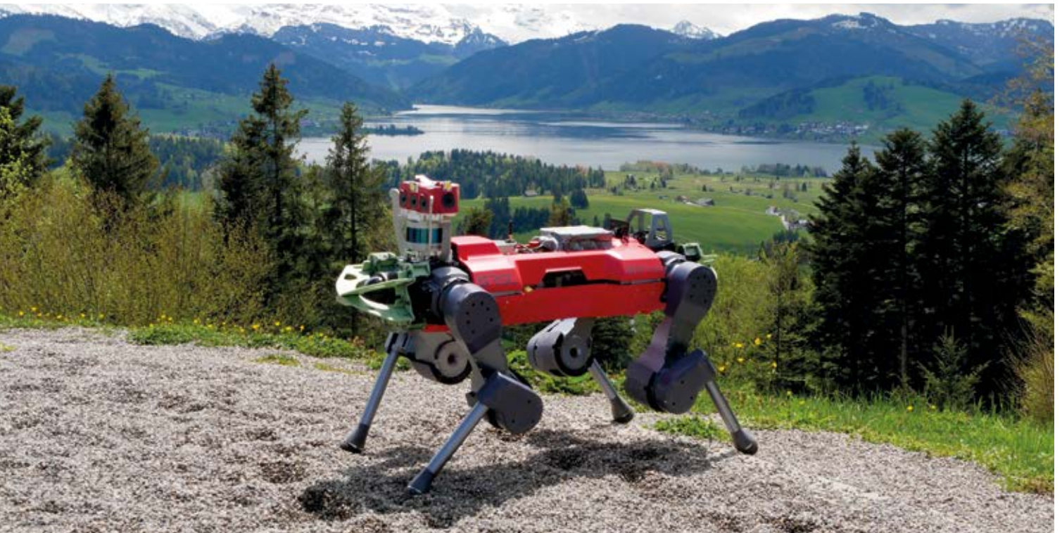
Quadrupedal robot ANYmal developed at ETH Zurich on the stony trail leading up to 1,098-metre-high Mount Etzel. (Image: Takahiro Miki)
