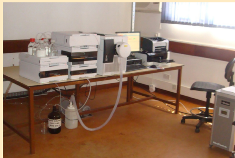
The LC-MS machine used to determine levels of aflatoxin contamination in maize at icipe, Nairobi Photo: Duncan Onyango Mbuge
