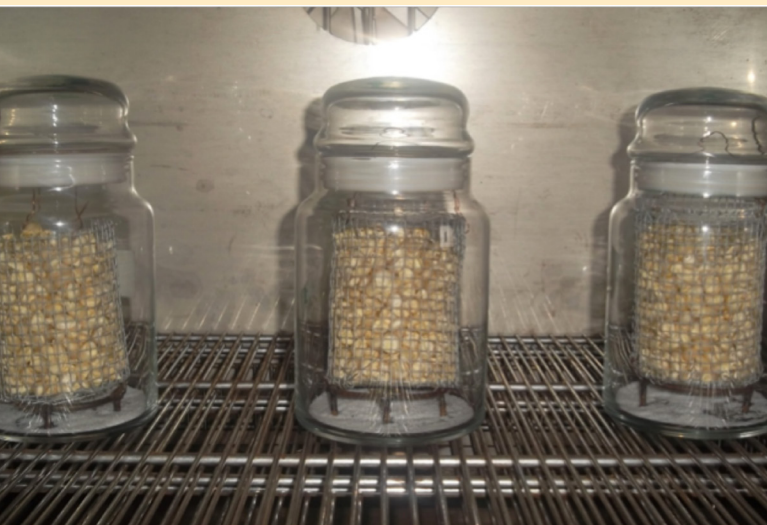
Super-absorbent polymers (powder at the bottom of the bottles) used to dry maize in an enclosed environment Photo: Duncan Onyango Mbuge
