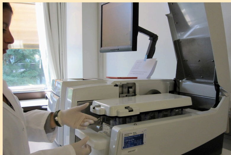
A 454 sequencing specialist preparing the machine for a sequencing run Photo: S. Henson
