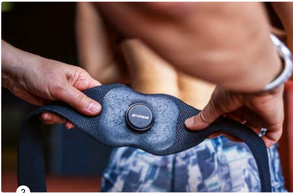
2 Sensors incorporated in a belt record the athlete's movements.
