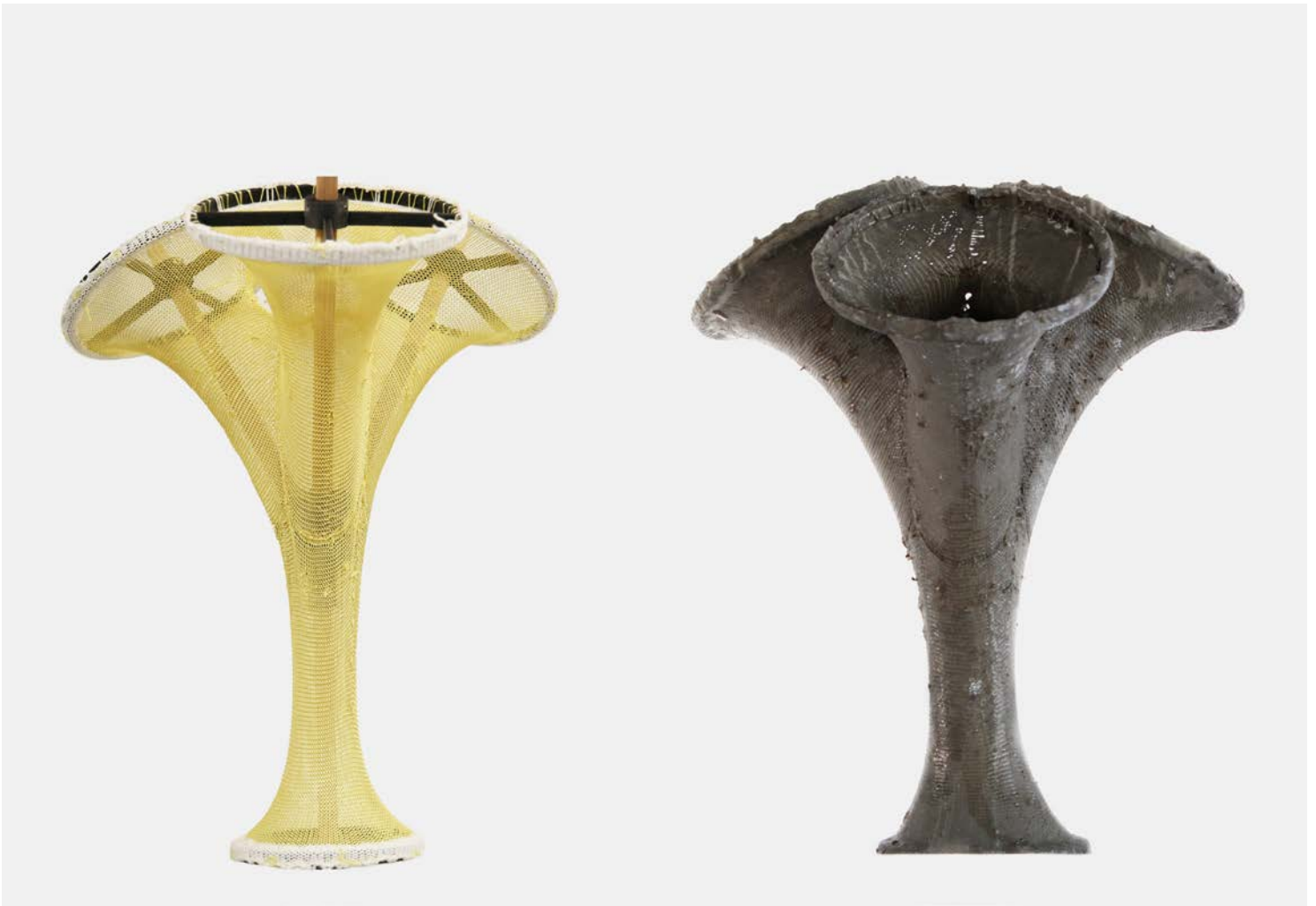
Mariana Popescu: KnitCrete: Stay-in-place knitted fabric formwork for complex concrete structures, 2017 [Chair of Architecture and Structures]
