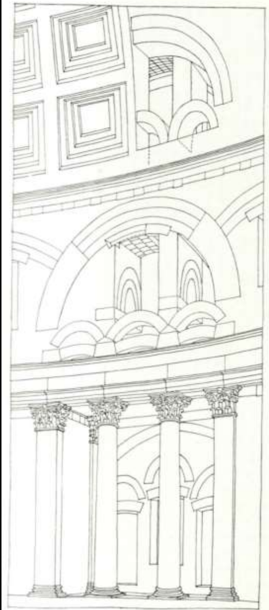
FIG. 110. Pantheon: Drawing of the structural principle in a division of the wall of the rotunda.
