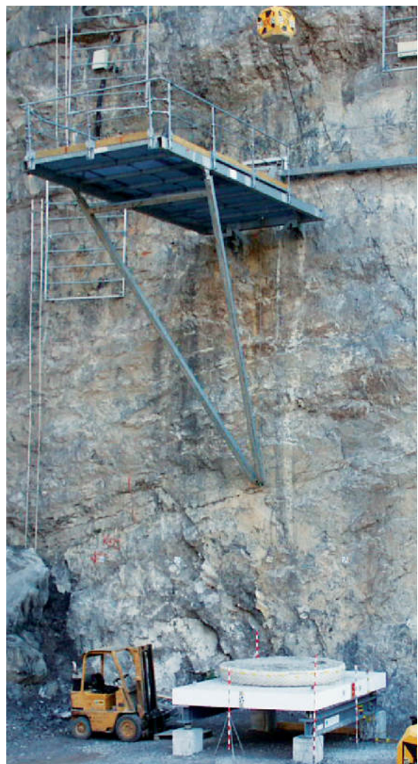
Fig. 34: A bolder of 800 kg is dropped on a reinforced concrete slab from 15 m of height.
