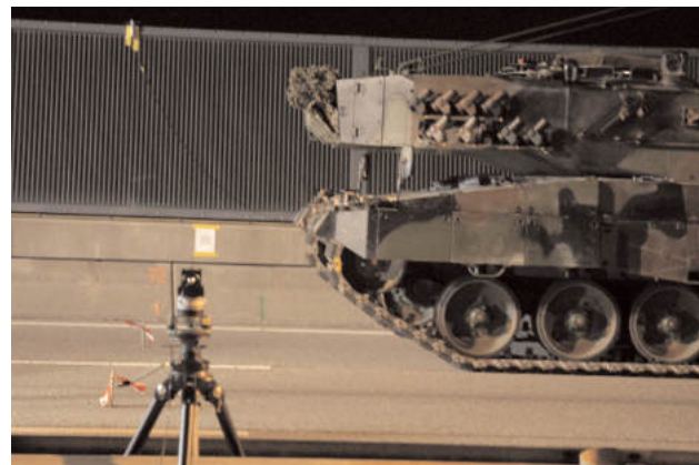
Fig. 10: Direct observation of cantilever slab deformations.
