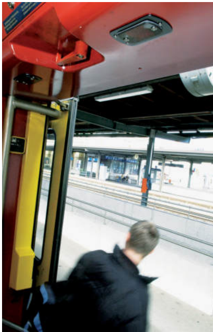
Fig. 45: Direction sensitive infrared sensors of the automatic passenger counting system (AFZ) of the Swiss Federal Railways (SBB).
