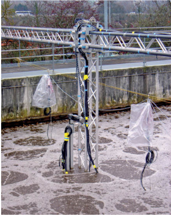
Fig. 1: Monitoring system for flow velocities (Acoustic Doppler Velocimetry, collaboration with VAW) and continuous ammonia detection system.
