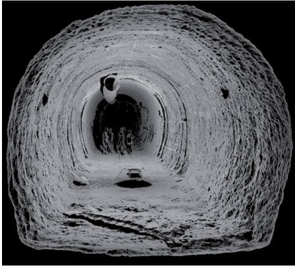
Fig. 1: Laser scanner point cloud: Because there is no air-placed concrete the rock structures are visible. Volume changes can be detected by comparison with later scans.
