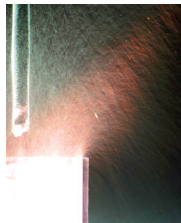
Fig. 4: «Granular fountain». Glass particles are violently ejected out of the jar by electro-static forces after they were charged only by pouring them through an acrylic tube. (FKW, HJH, T. Shinbrot)
