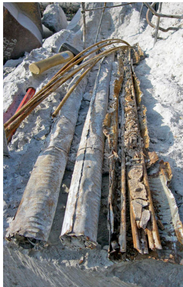
Fig. 4: Opened tendon with insufficient grouting.
