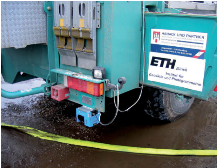
Fig. 1: Setup of the 2D laser scanner on the crane
