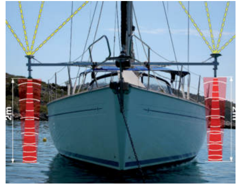
▲ Fig. 2: The measurement system combines GPS measurements (yellow) with ultrasonic ranging measurements (red/white).
