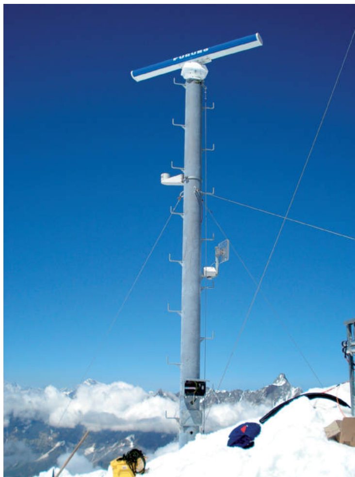
Fig. 4: The X-band radar installed on the Kf. Matterhorn.
