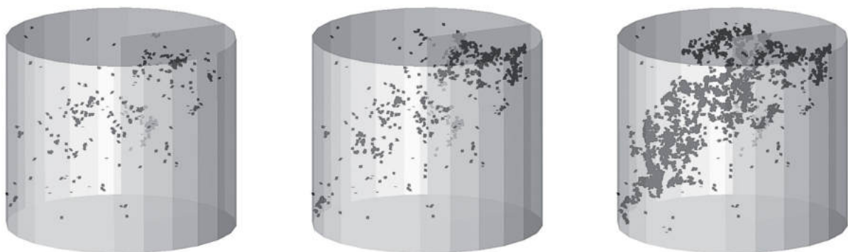
Fig. 4: Three-dimensional crack patterns at different stages.
