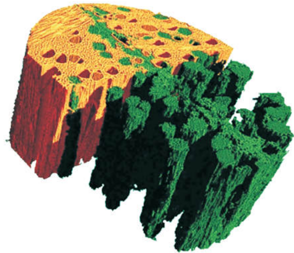
Fig. 2: Adhesive penetration into wood (reconstruction of synchrotron data set).
