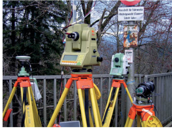
Fig. 2: Besides traditional surveying instruments like GPS-receivers or tachymeters, unconventional self-made constructions were installed, such as the web camera in the lower right. The use of diverse instruments allowed an insight into the possibilities and limitations of the equipment.
