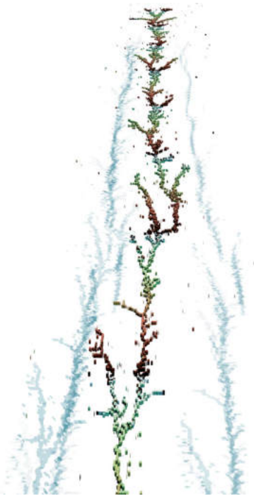
Fig. 7: Dynamic model fracture with severe crack branching simulated via a moving lattice method. Colours represent breaking time intervals. (FKW, HJH)
