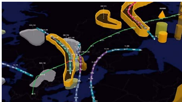
Turbulence ahead: A result of a master thesis at ETH Zurich that visualises aviation weather in 3D with the ArcGIS API for JavaScript 4.x for interactive exploration during pre-flight preparations by pilots
