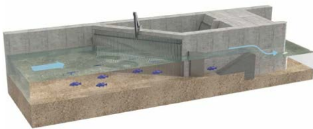
A safe guidance system for fish: a specially designed bar rack effectively guides downward migrating fish past the turbine, only slightly limiting the power plant's operations.
