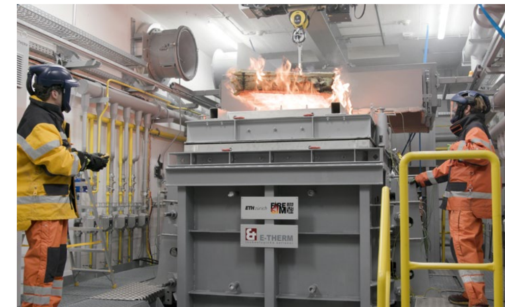
🕒 After 90 minutes the wooden piece is removed from the furnace and extinguished.
