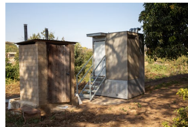
↑ The "Autarky" toilet developed at Eawag (right), shown here in a field test in Durban, South Africa next to a dry toilet. Autarky treats the three separate streams – water, urine and faeces – in situ.
