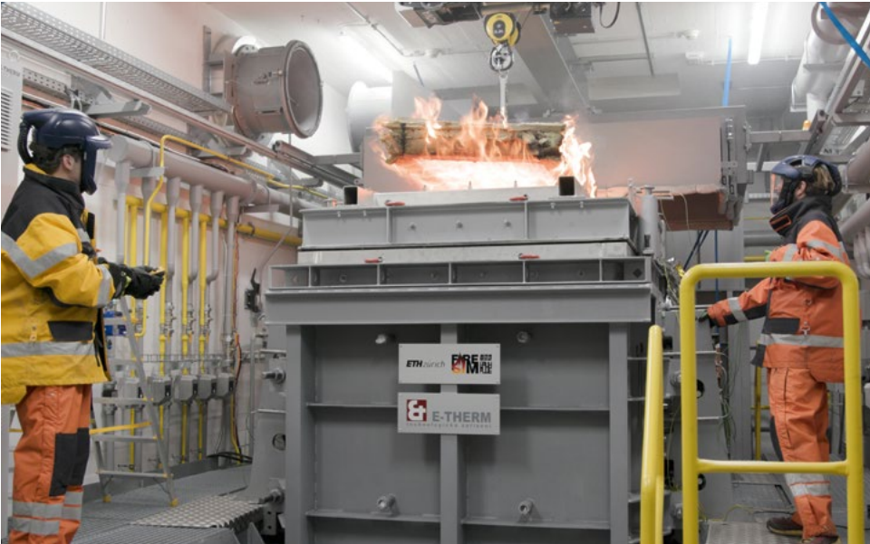
⌚ After 90 minutes the wooden piece is removed from the furnace and extinguished.
