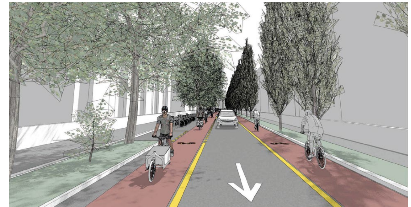
➦ In the E-Bike City , the urban road network for cars consists largely of one-way streets, whereas two-wheelers have dedicated lanes for both directions of travel.
