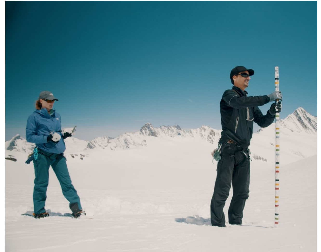
Daniel Farinotti and doctoral candidate Jane Walden install a mass balance stake at Grosse Aletsch glacier.
