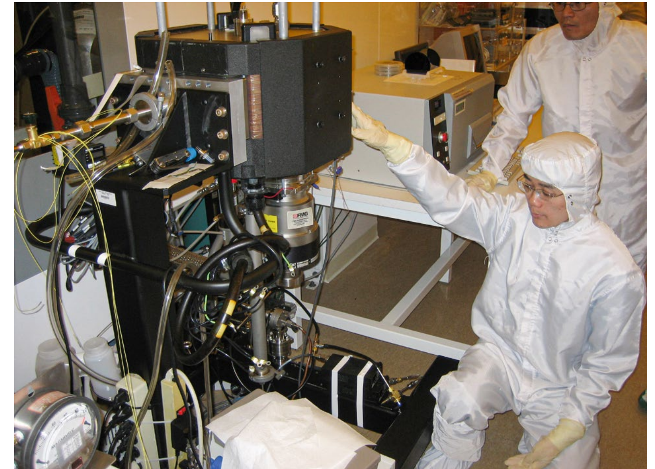
Jing Wang demonstrating a vacuum system for nanoparticle deposition on photomasks in a cleanroom.
