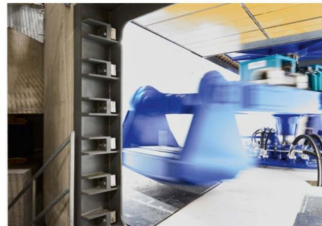
👉 The centrifuge is still rotating very slowly here. When it runs at full power, the doors are closed. The experiments it can carry out include testing the impact of an earthquake on certain soils.
