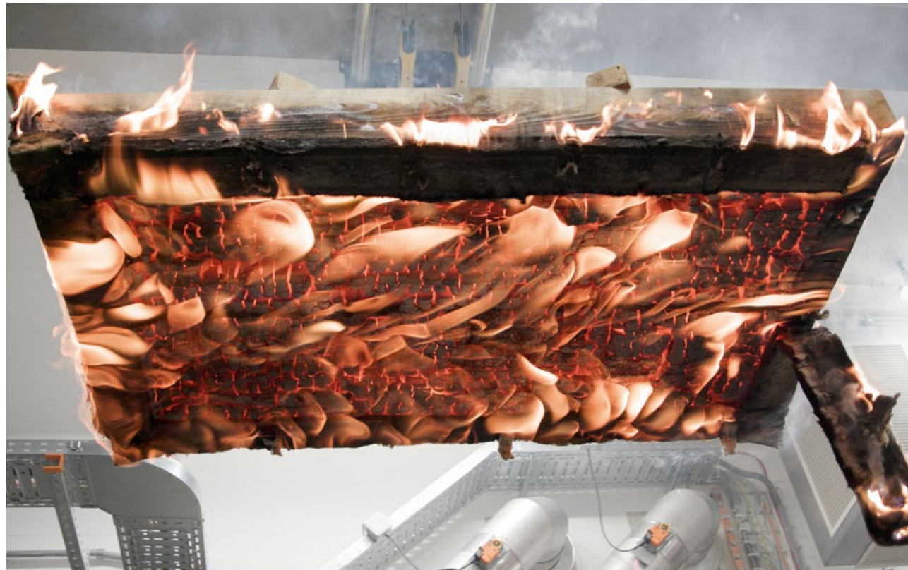
🔥 Fire simulator to test timber components for the construction of buildings.
