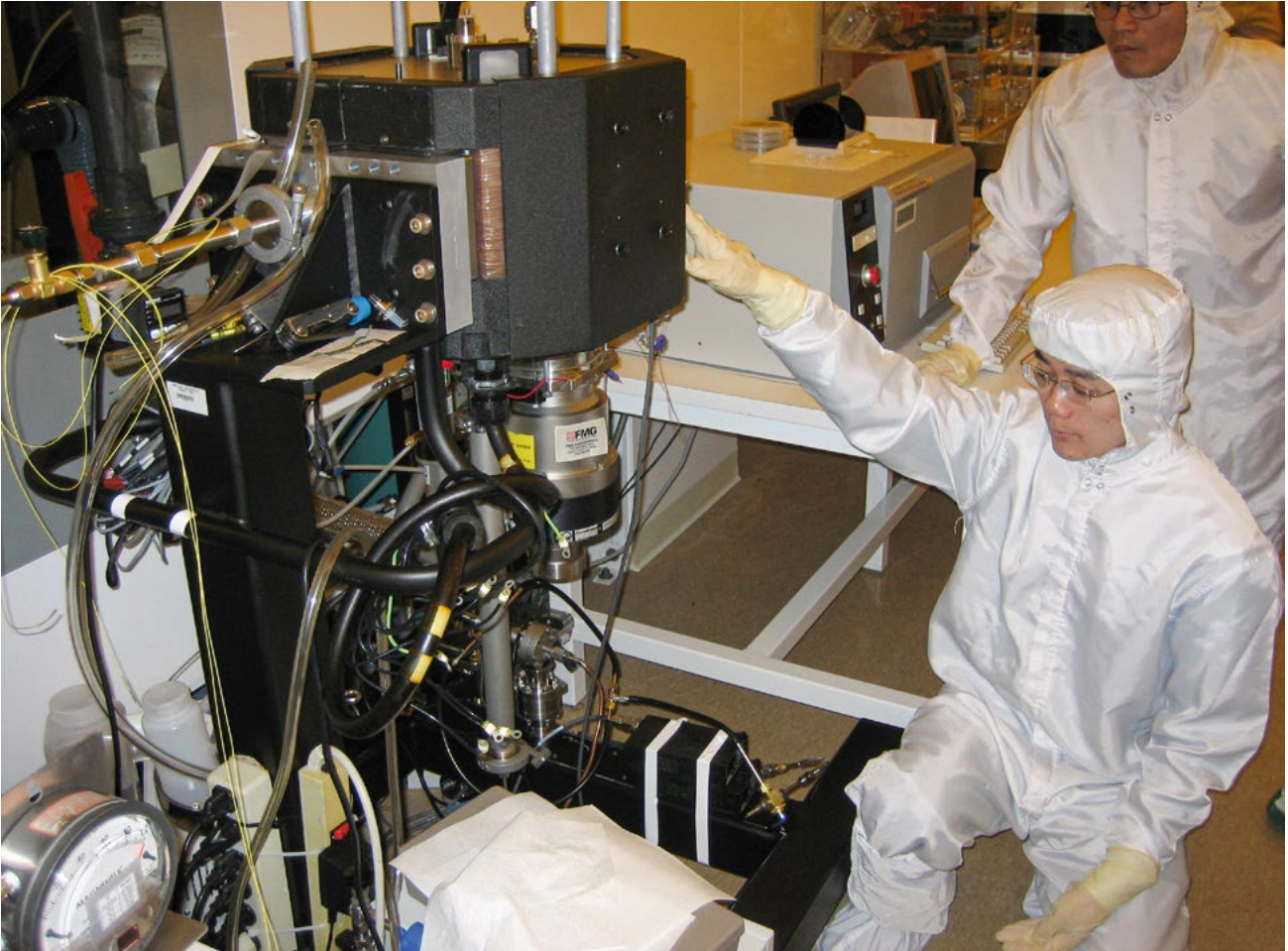
↑ Jing Wang demonstrating a vacuum system for nanoparticle deposition on photomasks in a cleanroom.
