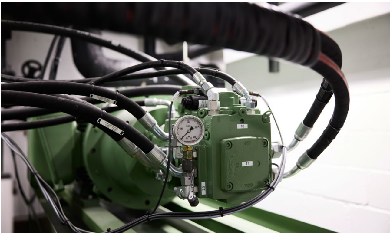
↑ The oil pumps drive the centrifuge and make an immense racket – they run at 1.000 hp.
