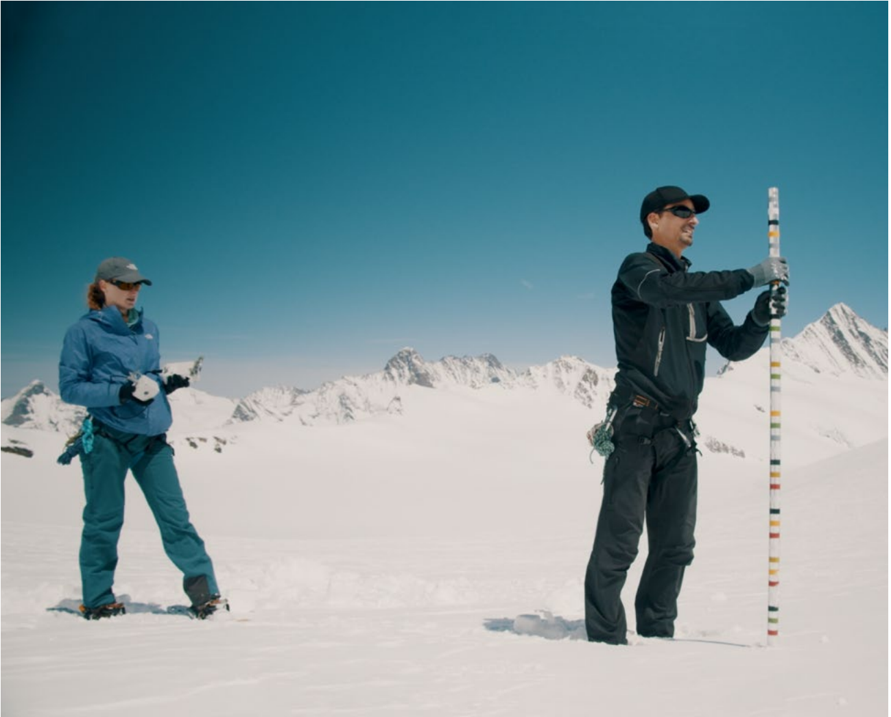
↑ Daniel Farinotti and doctoral candidate Jane Walden install a mass balance stake at Grosser Aletschgletscher.
