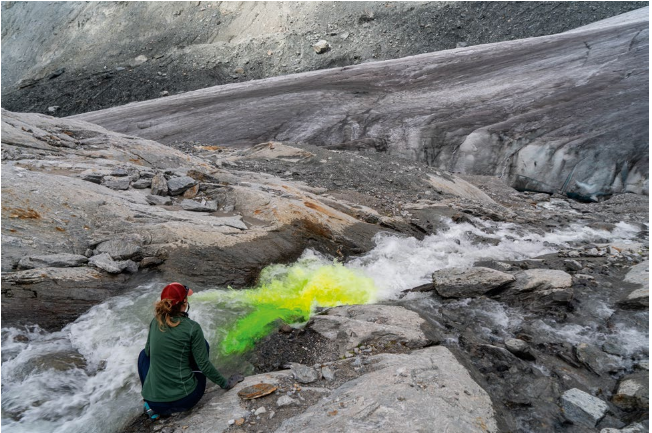
⬆️ One of the prize-winning photos in the SNSF Scientific Image Competition 2024: "Follow the water" by Leo Hösli (MSc Student D-BAUG). The image shows a tracer experiment near the Findel glacier in Valais.
