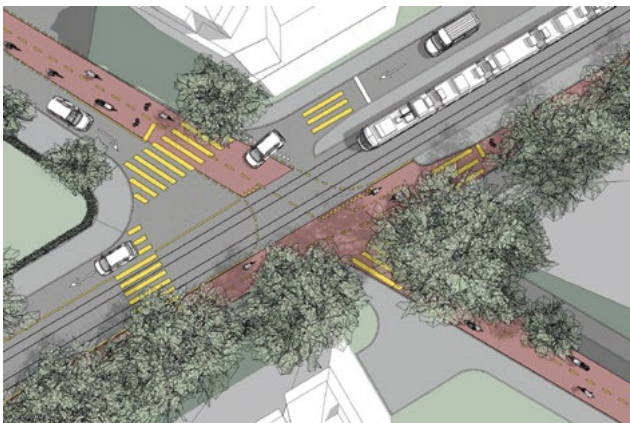
↑ View of an intersection in the E-Bike City: Two-wheelers will have their own double lane and public transport will have its own lane as well. Cars drive on one-way streets.
