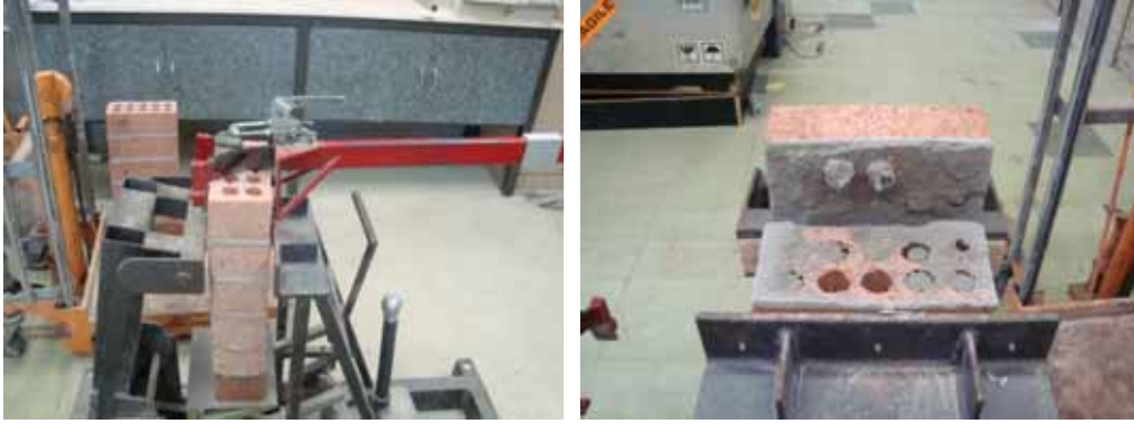
Figure 5: Bond wrench test apparatus and joint failure
