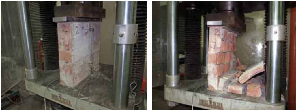
Figure 9: Compression test on cut-out specimen and its failure
