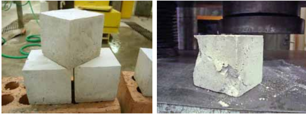
Figure 3: Mortar test cubes and typical failure
