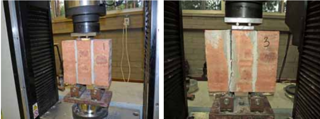
Figure 7: Shear bond test apparatus and shear failure
