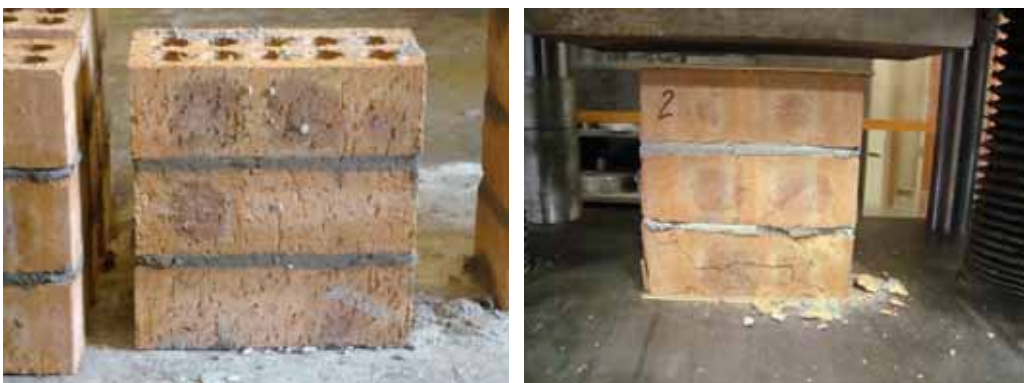
Figure 8: Compression test on a masonry triplet
