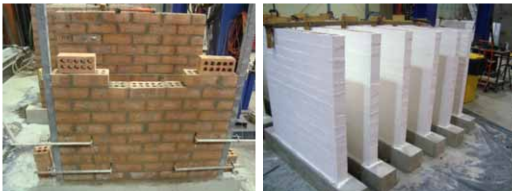
Figure 11: Construction and completion of wallette specimens
