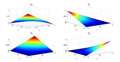
$$\mathbf{K^{tot}} \cdot d = f^{tot} \quad \text{where} \quad \mathbf{K^e} = \int_{\Omega^e} \mathbf{B}^T \mathbf{D} \mathbf{B} d\Omega, \quad f^e = \int_{\Omega^e} N^T B d\Omega + \int_{\Gamma_T^e} N^T t_s d\Gamma$$
