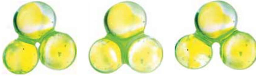
Fig. 7 (left) Three grains with liquid bridges, (center) trimer with filled pore throat and (right) ruptured trimer with subsequent liquid redistribution.
