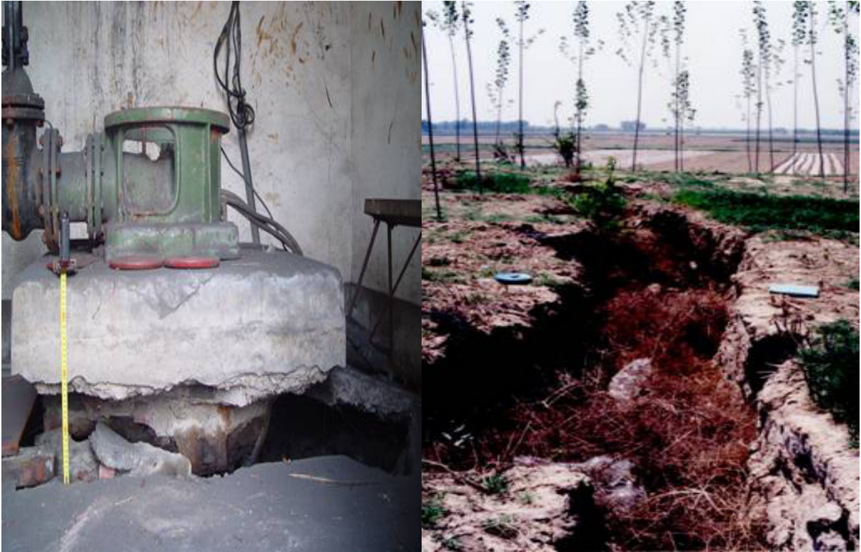
Figure 7: Overpumping of the deep aquifer destabilizes the ground and eventually leads to a collapse of the clay layer, which causes land subsidence (left picture) and ground fissures (right picture) [2].
