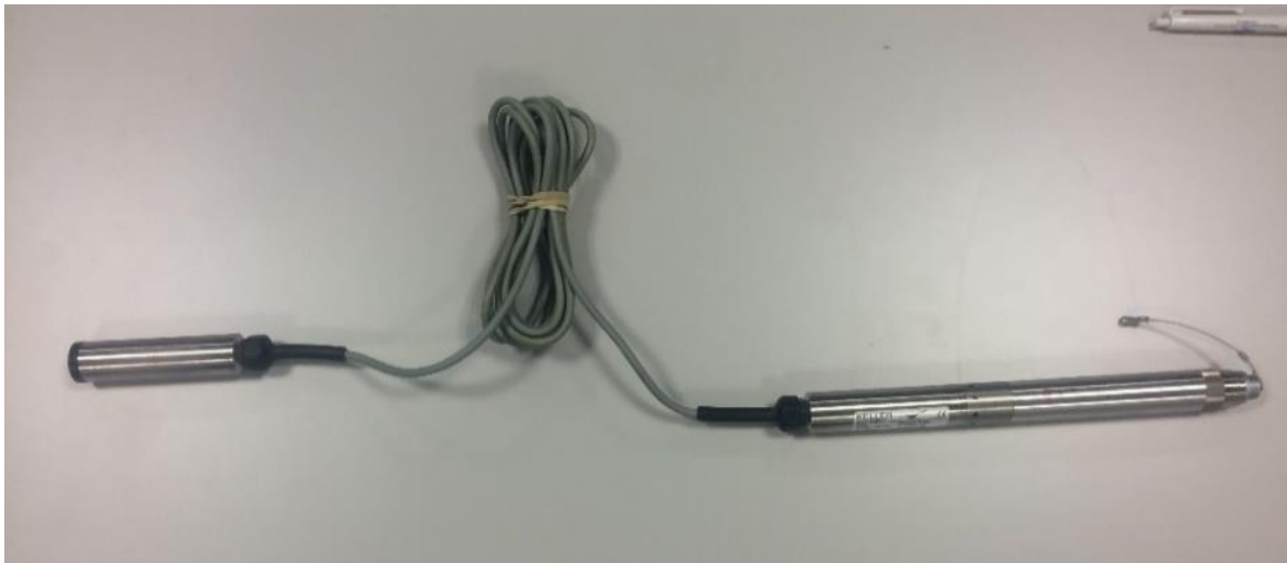
Figure 5: The logger. The left sensor is submerged, the right sensor is placed above the water surface (contains the internal memory and the interface to read the data).
