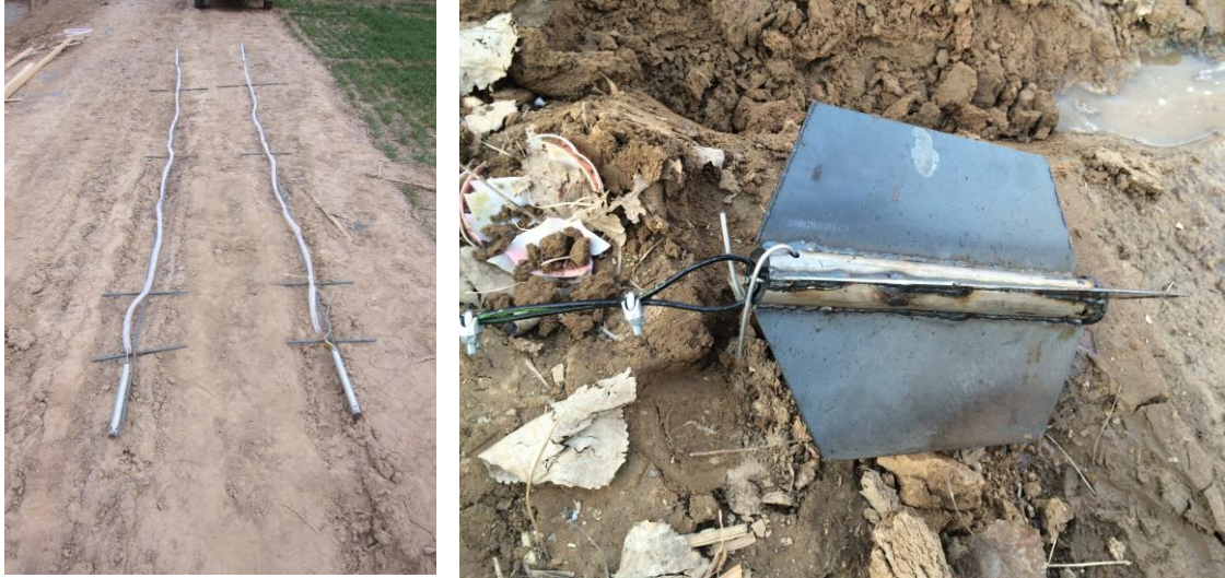
Figure 7: The sensor structure. Left: the entire structure for lake sensors. Right: the anchor for the river sensor.
