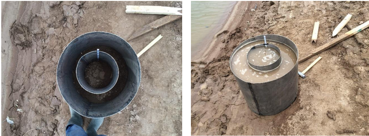
Figure 8: double-ring infiltrometer test. Left: the infiltrometer setup seen from above, before the start of the experiment. Right: the infiltrometer working on-site.
