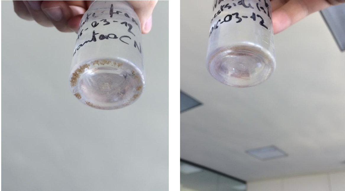
Figure 15: Water samples from the canal (left) and from Lake 1 (right). The pictures were taken more than two month after sealing, when particles already flocculated. The turbidity is higher in the river than in the lake, as visible by the size and number of flocculated particles.
