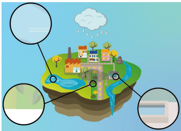
Fig. 1. Sponge city schematic. Blue-green infrastructure treatment systems capture urban stormwater and can remove selected pollutants.
