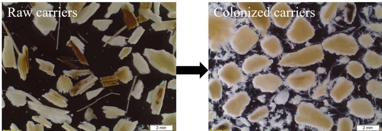
Preliminary reactor operation showing colonization of biomass on the organic kenaf carriers after 49 days.
