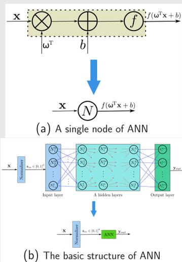
Figure 1: Schematic view of a single node and the layered structure of a BPNN
