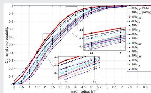
Figure 4: Cumulative probability of positioning error for BPNN-LA
