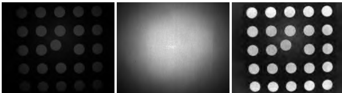
Figure 3.6: Processing of amplitude images of the photogrammetric calibration test field from the SR-3000 in order to reduce the decreasing amplitude with an increasing radial distance from the center of the image: original amplitude image (left), blackboard image (center), and the processed image for use in further analysis (right).
