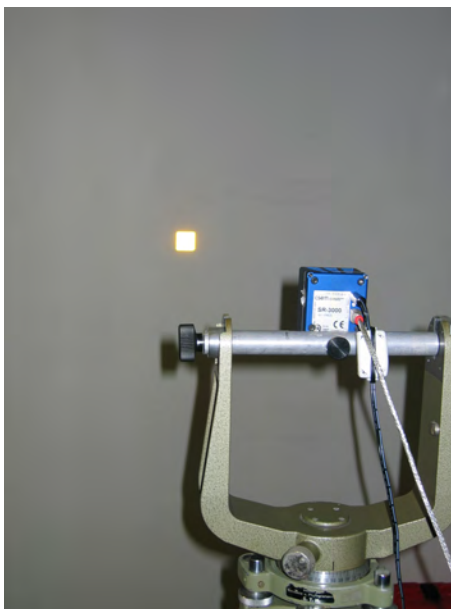
Figure 3.56: Fixed-Pattern Noise experimental setup for the SR-3000. The sensor is mounted on a tripod on which the total station has been placed before. The total station was used to determine the perpendicular projection of the camera position on the white wall. The SR-3000 then is oriented with respect to the optical center of the sensor towards the wall.
