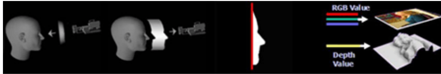
Figure 2.35: Depth keying principle. A scene is illuminated with a light pulse. The incoming signal is captured only for a short period of time. The impinging optical energy then is related to a specific distance within this interval. Thus, the chopping of the time domain leads to distance interval mapping, sequentially.
