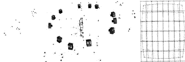
Figure 3: Recovered camera poses and 3D coordinates of the tie points (left). The influence of the APs on the image grid, 3 times amplified (right).
