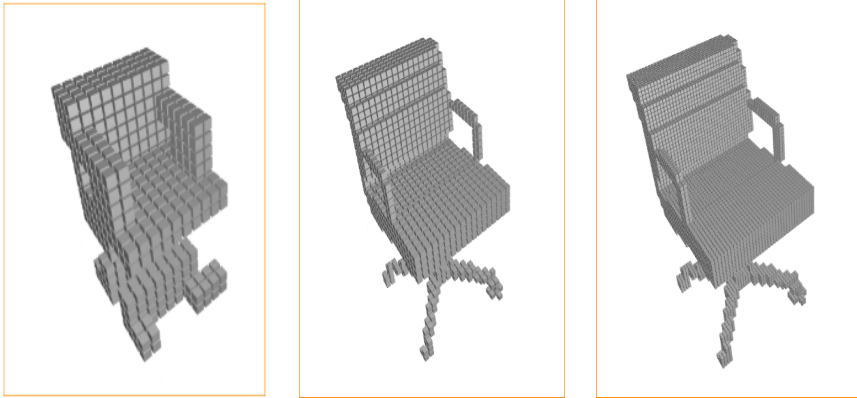
Figure 3.1: Example of the built-in voxelization method applied to a chair. The number of voxels per cm increase from left to right.
