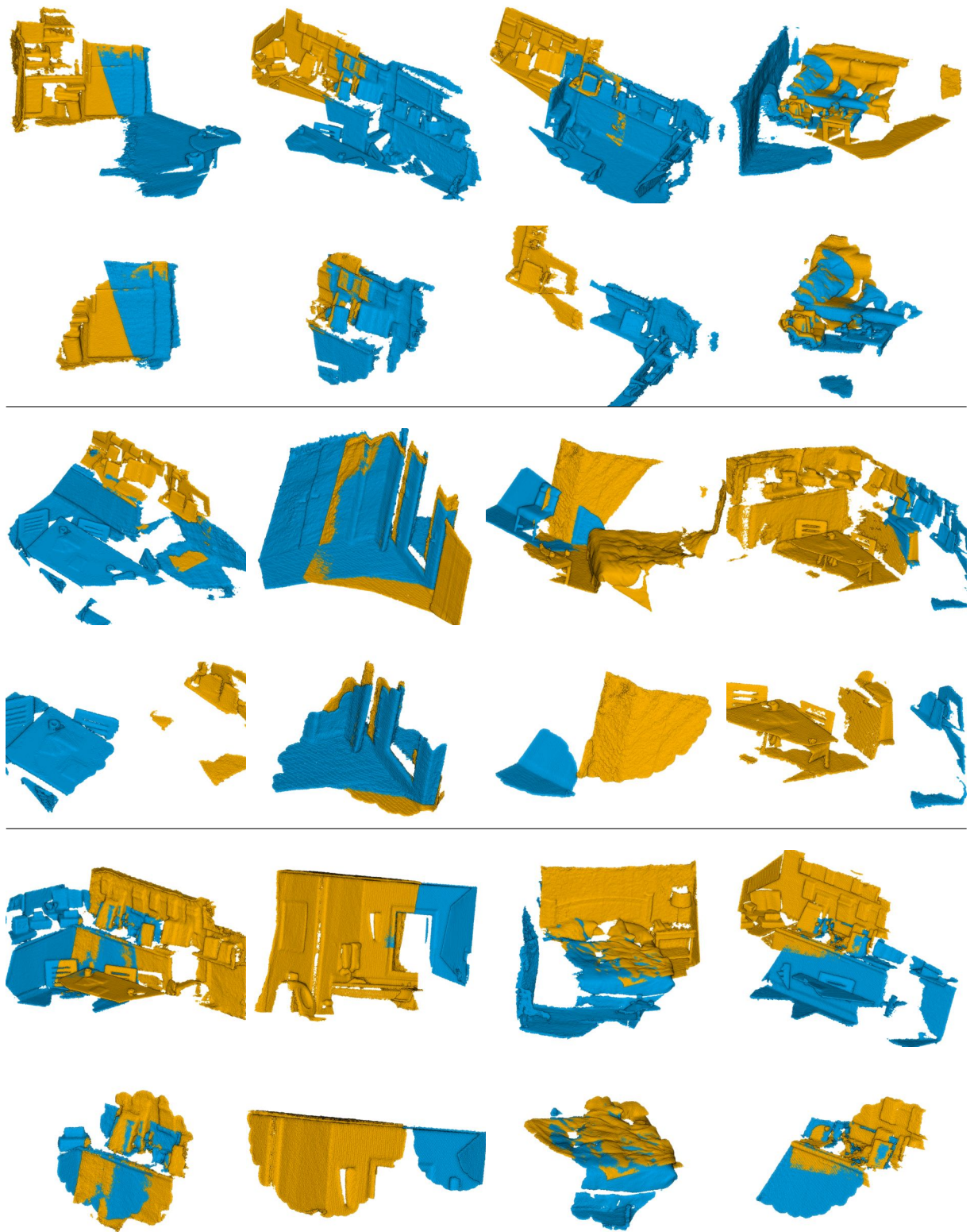
Figure A.2.: Visualisation of intermediate pruning results on LowOverlap benchmark. We randomly sample 12 fragment pairs, the first row shows the input, the second row shows the pruning results. Note that each patch actually only has 512 points, for better visualisation, we apply a radius search to the raw point clouds to get dense representation.
