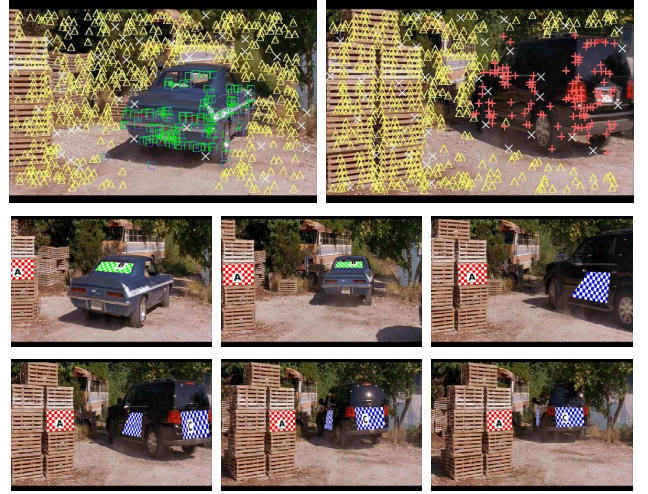
Fig. 4. Car sequence. Top: segmentation results (operations: initial segmentation, motion termination, new motion detection). Bottom: 3D augmentation.
