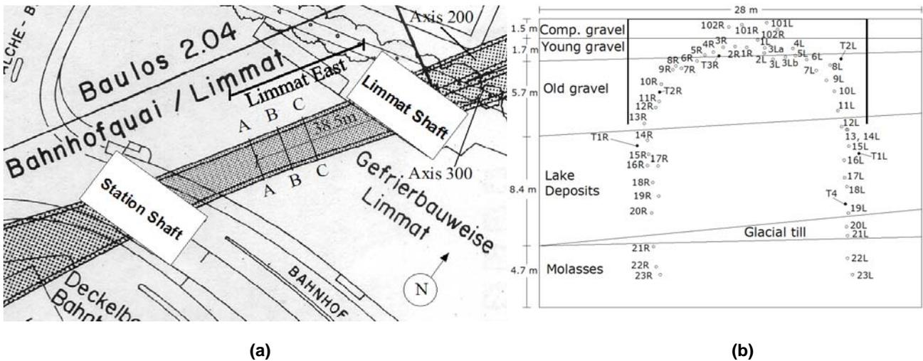
Fig. 7 (a) Plan view of Limmat under-crossing [8] and, (b), cross section A-A with actual location of the freeze pipes and auxiliary measures
