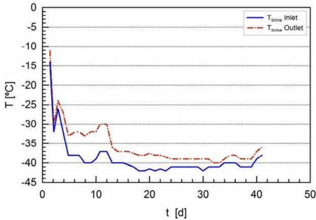
Fig. 2 History of the freeze pipe temperature
