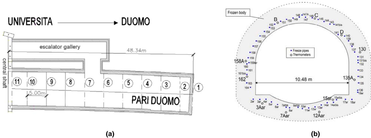
Fig. 5 (a) Plan view of the Pari Duomo platform tunnel and, (b), cross section 11 with freeze pipes and thermometers chains
