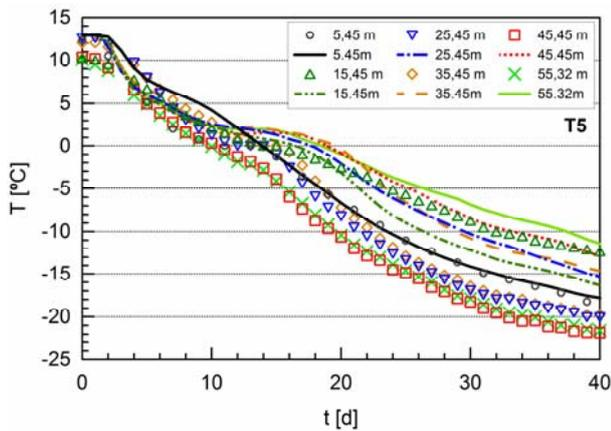
Fig. 4 Cooling history along the temperature sensor chain T5, positions measured from the working pit (symbols = measurements, lines = simulation results)
