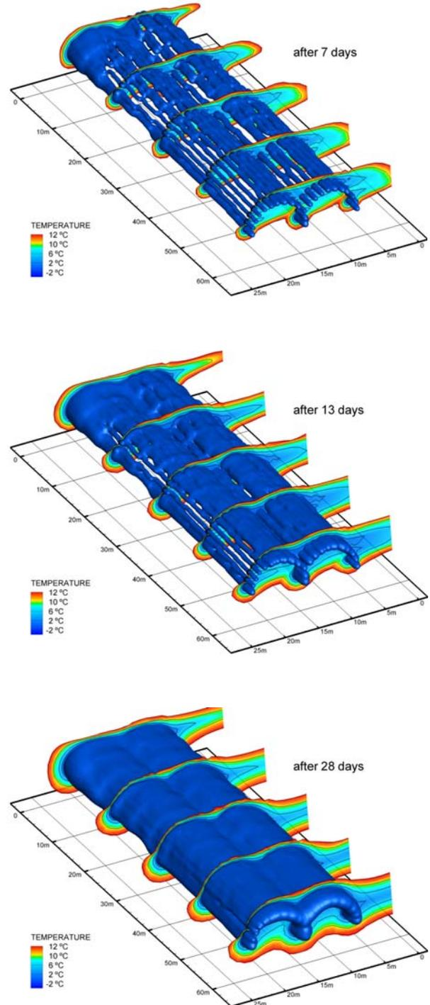
Fig. 3 Simulation results: longitudinal isothermal contour at  $-0\text{ }^{\circ}\text{C}$  (frozen body) and isothermal lines at 5 cross sections
