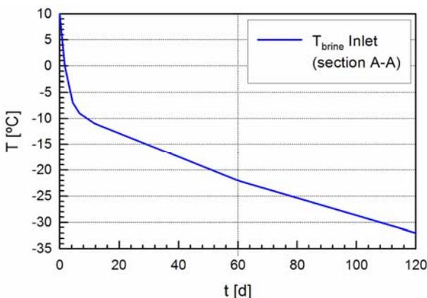
Fig. 8 History of the freeze pipe temperature
