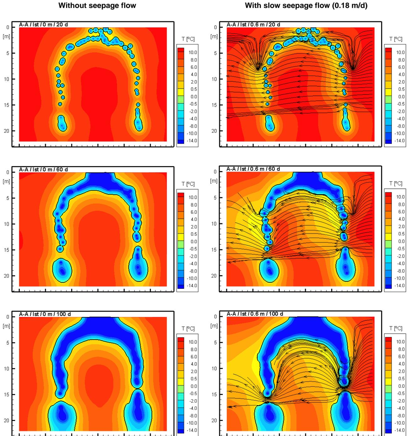
Fig. 9 Temperature distribution for the case without seepage flow (left) and with slow groundwater velocity (right) after 20, 60 and 100 days. The black contour line represents the extent of the frozen body (isotherm 0 °C) and the arrow curves selected streamlines
