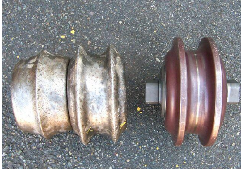
Figure 14. 14" Monobloc cutters as used on East Side CSO Portland
