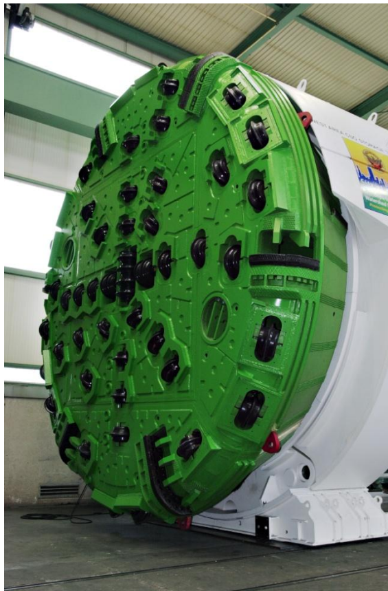
Fig. 15: TBM S-288 (S-289) 8,23m, 19" backloading cutterhead, West Area CSO Atlanta, USA
