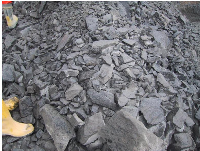
Figure 17: Typical tunnel muck showing crushed blocks from open mode operation
