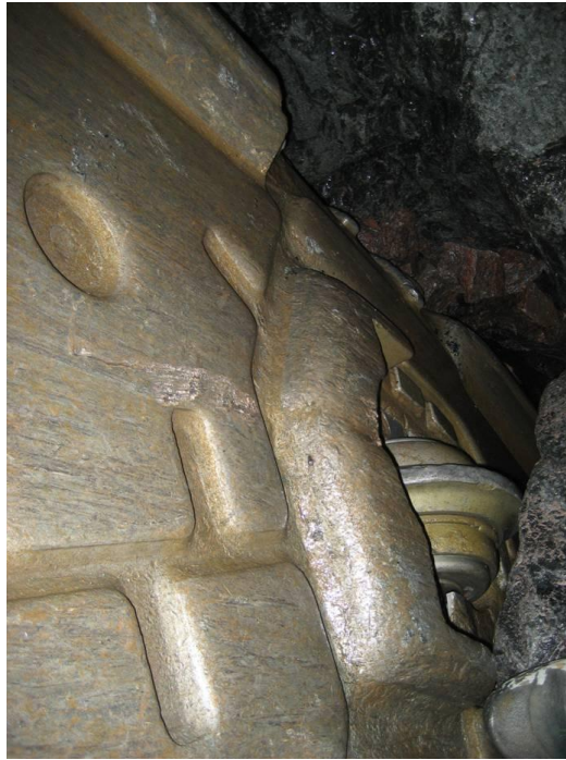
Figure 20: Front wear protection in worn conditions before replacement and repair
