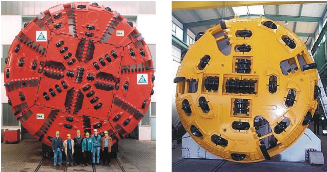
Figure 8. EPB cutterheads for variable ground: Porto Metro 2000 (left), Singapore DTSS 2003 (right)
