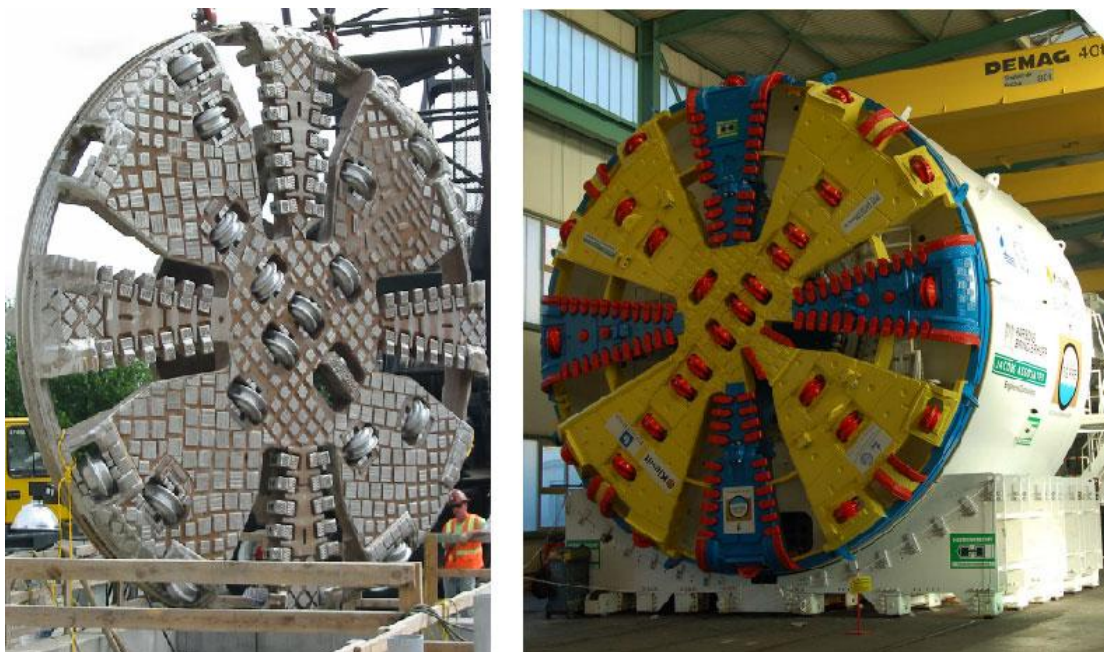
Figure 6. Modern STBM cutterheads: West Side CSO Portland (left), East Side CSO Portland (right)
