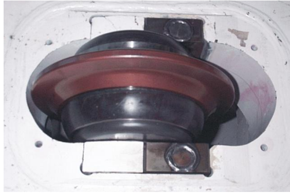
Fig. 8: modified cutterhead interface and housing design
