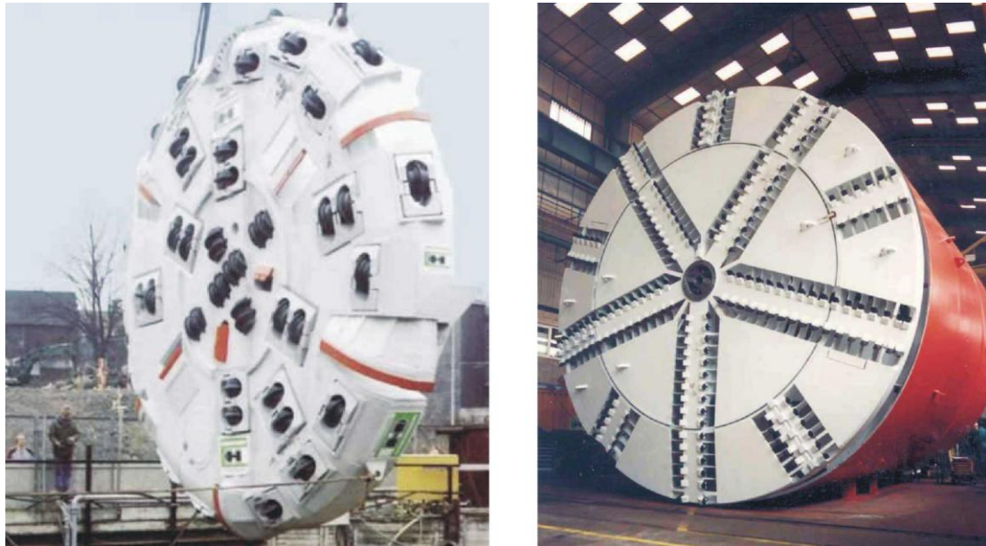
Figure 5. Early closed STBM cutterheads: Mülheim 1990 (left), Strasbourg 1991 (right)
