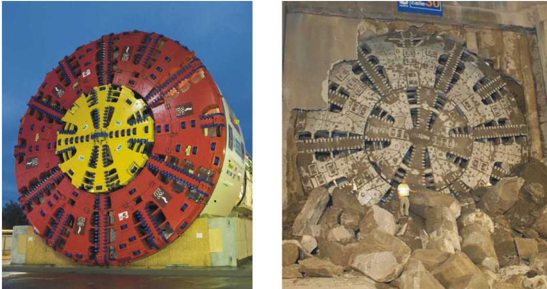
Figure 11. EPBM for M30 Madrid during shop assembly and in the arrival shaft
