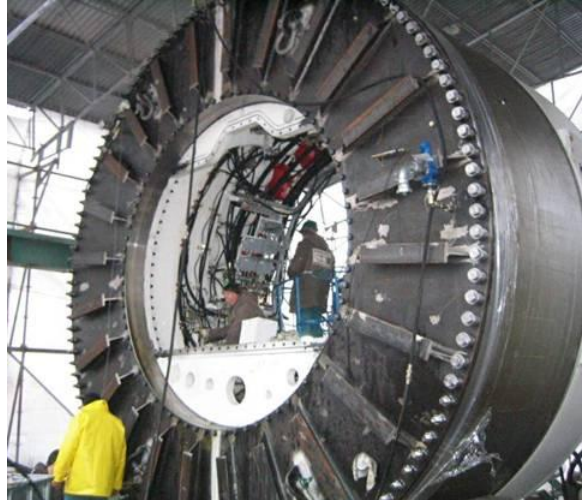
Figure 11: Original size shop test of the main drive seal system
