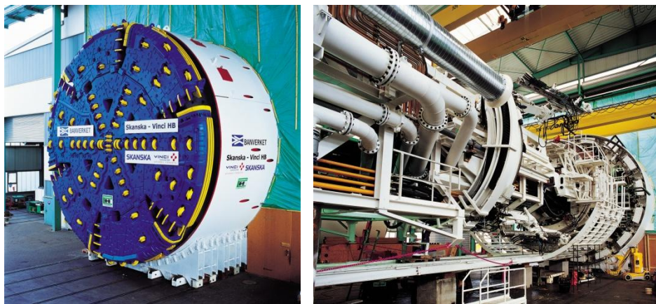
Figure 6 and 7: The S-246 Hallandsås TBM pre assembled in the workshop
