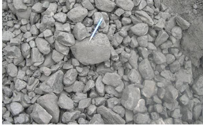
Figure 18: Typical tunnel muck from closed mode operation (rounded blocks)
