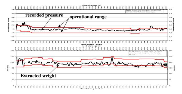
**The control of "face support pressure"** is necessary to ensure that the face stability is maintained during the EPBS advance but also during the stoppages. The support pressure is applied, within the excavation chamber (plenum), via the excavated and appropriately conditioned muck, by the pushing of the thrust jacks.
