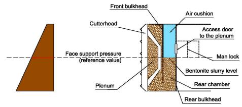
The following are the key excavation-parameter values to be measured on the Hydroshield (or Slurry Shield, like it is called generally today)
