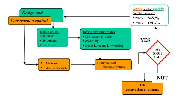
The control system activation gives real-time warnings to the process controllers, even before the threshold values are being exceeded, when their *trend* is showing a tendency to the limits, thus allowing the prompt adoption of counter measures.
