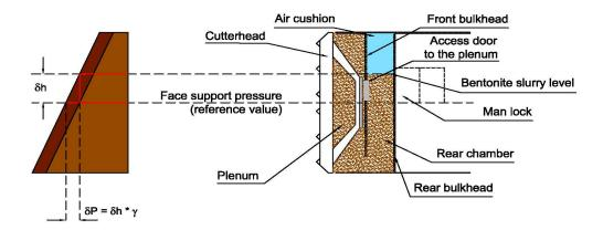
This could be a very dangerous situation as consequence of material entering into the chamber due to a face collapse. Another possible cause could be some difficulty into the discharge line (see next point).
