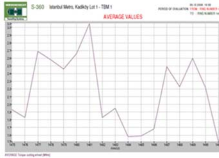
The decrease of torque due of stalling of disc cutters in blocky ground.
