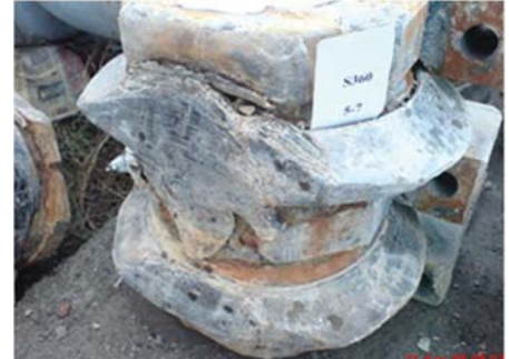
The wear of twin disc cutter due of stalling disc cutter in blocky ground.
