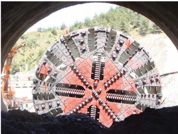
13.7 m diameter Single shield TBM
