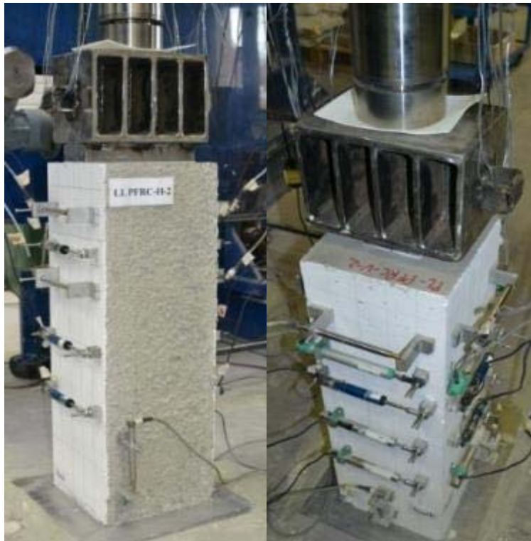
SMALL SCALE TEST reproducing the local behavior under TBM thrust jacks
