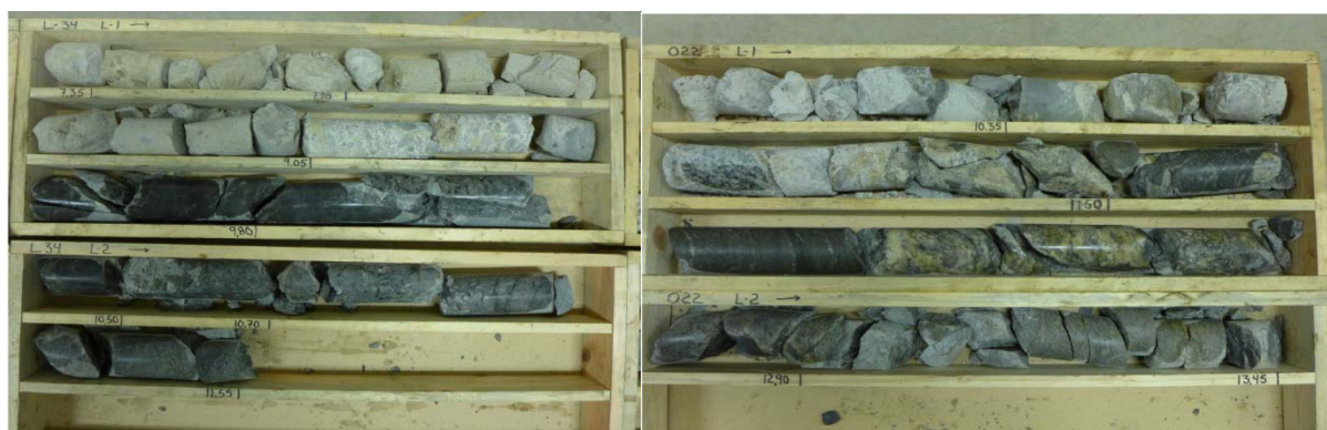
Figure 3. Core drilling of the grouted material and rock mass
