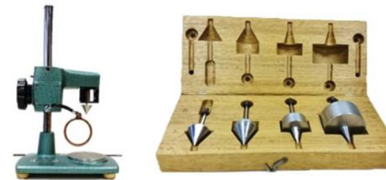
Figure 3. Fall cone test apparatus.
