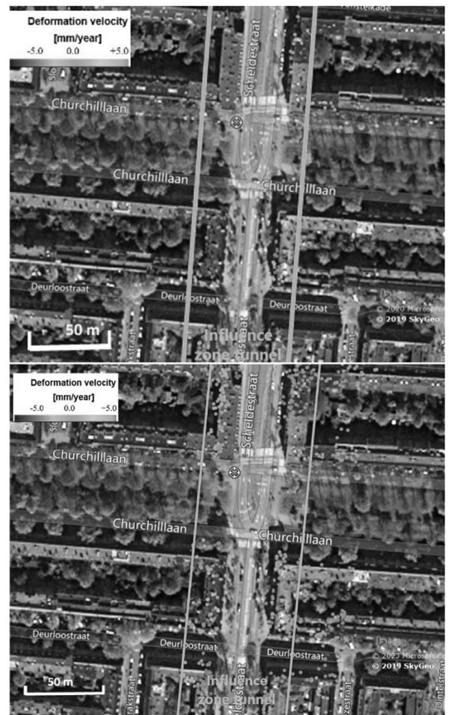
Fig. 9. InSAR points near Churchillaan : (a) low points, on the ground surface. (b) high points, on the buildings. The colored dots indicate the vertical deformation rates in mm/y. The yellow lines indicate the influence zone of the tunnel.
