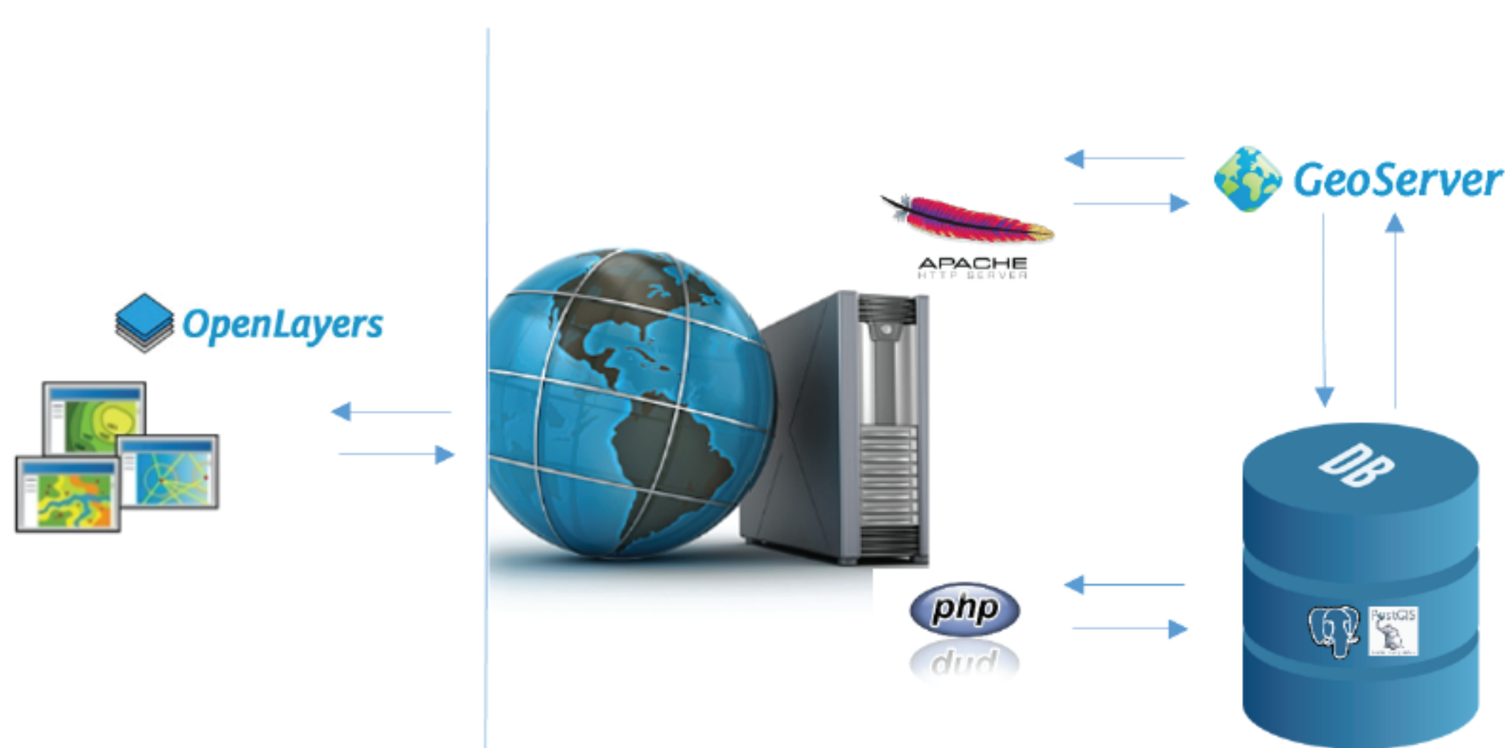
Figure 2: The infrastructure - three tier system architecture
