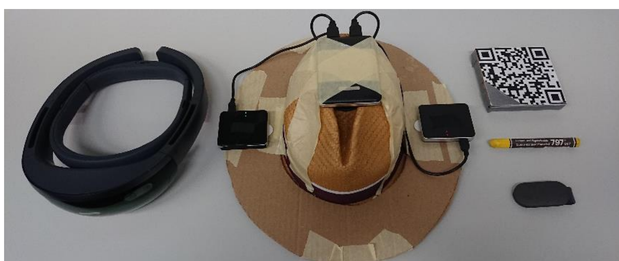
Fig. 1. Study material: HoloLens, Positioning system prototype, measurement marker, marking crayon
