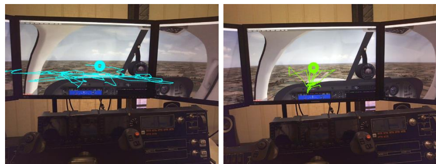
Fig. 2. Eye tracker data showing the scanpaths of participants looking for an object without the belt (left) and while wearing the belt (right).
