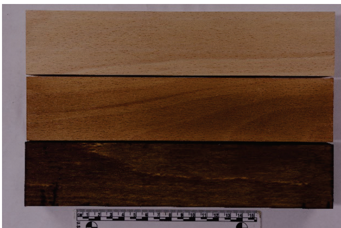
Figure 1: Specimens with a size of 5 x 5 x 25 cm 3 . Top: native beech sample; middle: Paraffin wax treated sample; bottom: pine tar treated sample.
