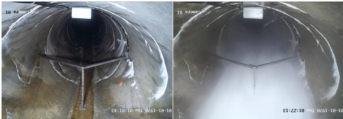
Fig. 3 Air-water flow instrumentation installed in the spillway tunnel (left); measurement of air-water flow properties at a flow velocity of roughly 40 m/s (right). View in flow direction (photos: B. Hohermuth, VAW).
