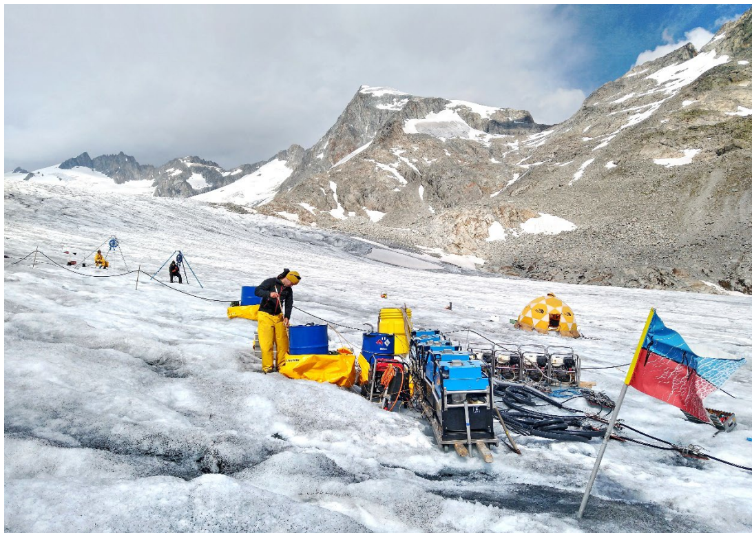
Fig. 27 Hot water drilling at Rhonegletscher in the Kanton Valais. Credit: Dominik Gräff.
