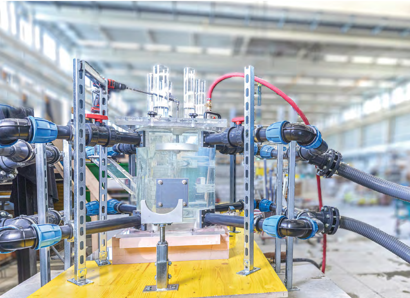
Fig. 4: Laboratory setup designed for sensor investigations to measure suspended sediments up to the size of coarse sand.
