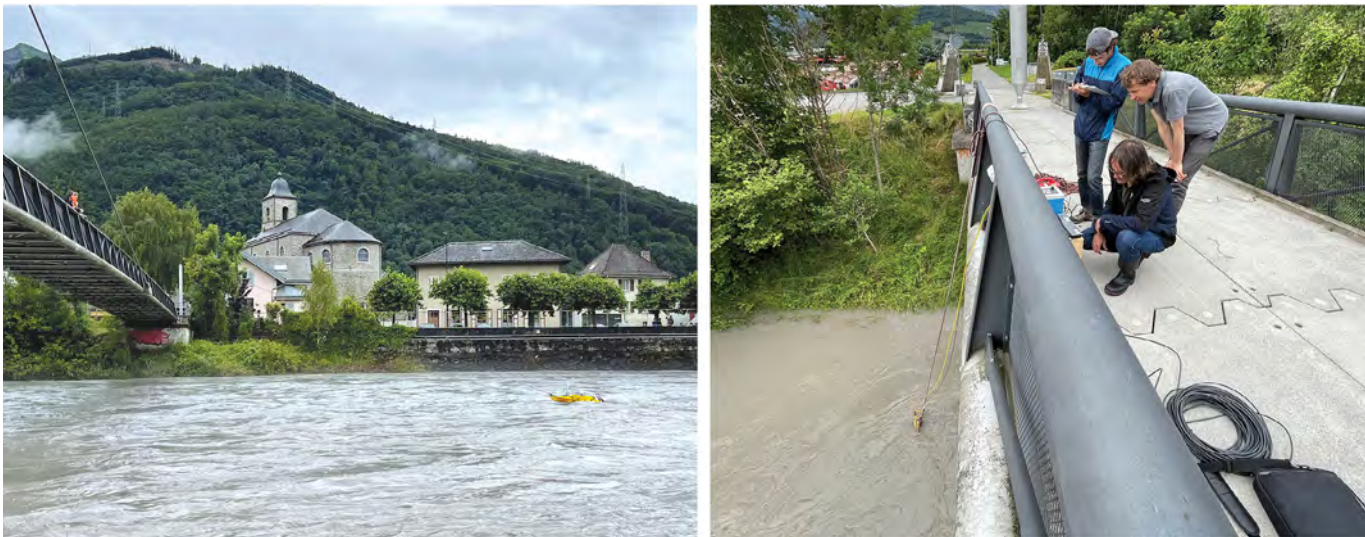
Fig. 33: Field velocity (left) and suspended sediment (right) measurements in River Rhône near the town of Bex conducted by VAW in the scope of Work Package 4 of HydroLEAP. The field data are used to evaluate the sediment abrasion potential for the turbines of the planned new HPP Massongex-Bex- Rhône.
