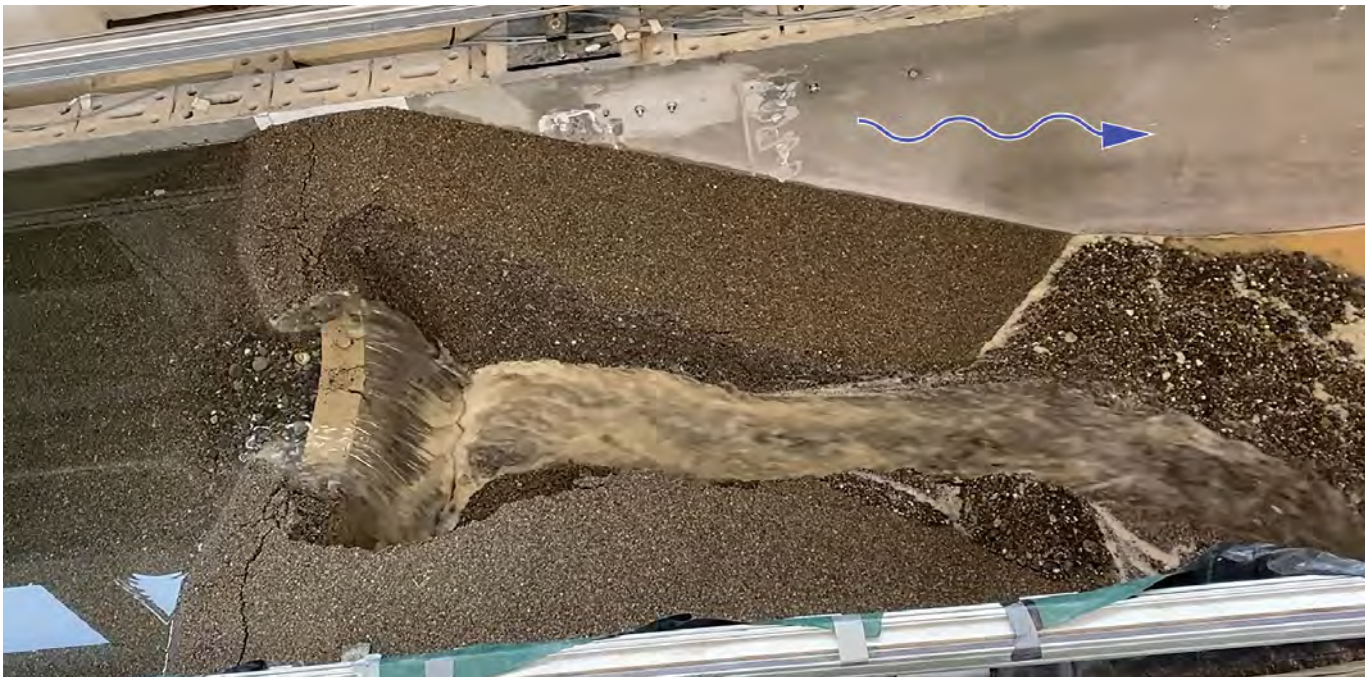
Fig. 16: Experiment of zoned dam failure due to overtopping, just prior to failure of the core. Blue arrow shows flow direction.
