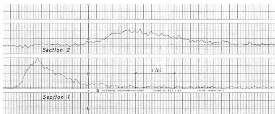
Fig. 9 Time series plot of conductivity between flume electrodes as slug of salt solution passes.
