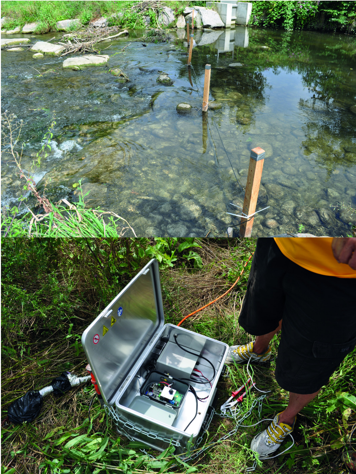
Figure 6.4 Equipment for the field tests. Top: stationary antenna stretched over the river width (water flows from right to left); bottom: tuner box with standard remote tuner board placed besides the river.
