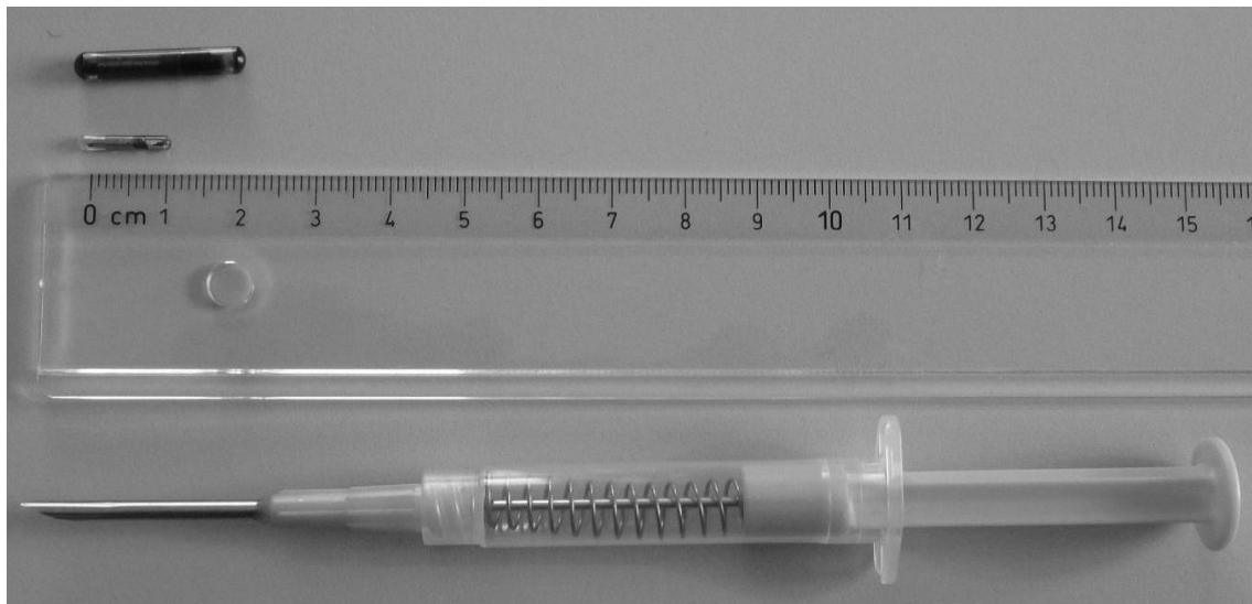
Figure 6.1 PIT tag equipment with large (23 mm) and small (12 mm) PIT tags and needle.
