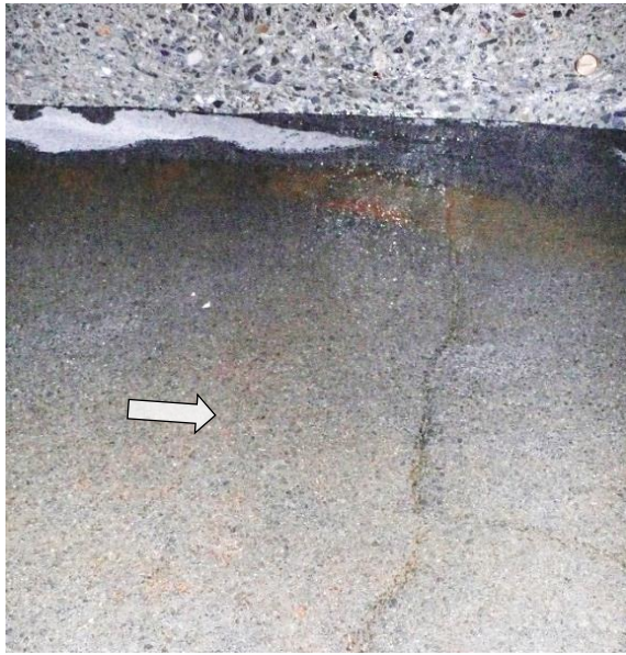
Figure 11: Crack in the HPC test field running perpendicular to the flow direction, picture taken 2012
