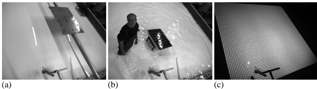
Fig. 3.11 Shots by camera 1 of (a) orientation measurement; (b) calibration measurement; (c) measurement of experimental run
