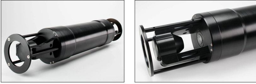
Figure 8: Laser in-situ scattering and transmissometry (LISST) 100X Type C (left) and detail of the instrument's head with laser and ring detectors (right) [Images from Sequoia Scientific, Inc. ]
