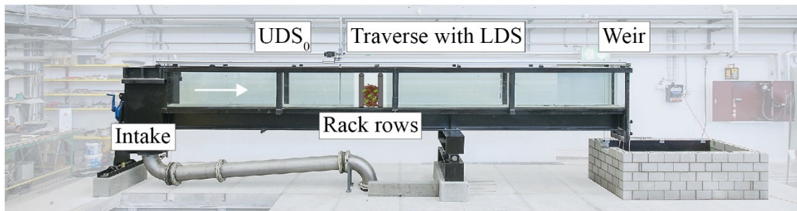
Figure 4.5 Photo of model flume II (small flume) at VAW with LDS = Laser Distance Sensor and UDS = Ultrasonic Distance Sensor
